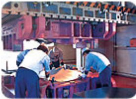
Ogihara personnel remove a tryout operational panel from the die for dimensional measurement using Optigo. Source: CogniTens
